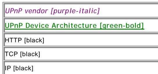
At the highest layer, the presentation page is specified by a UPnP vendor. Moving down the stack, the UPnP Device Architecture specifies that this page be written in HTML. The page is delivered via HTTP over TCP over IP. For reference, colors in [square brackets] are included for consistency with other clauses in this document.
