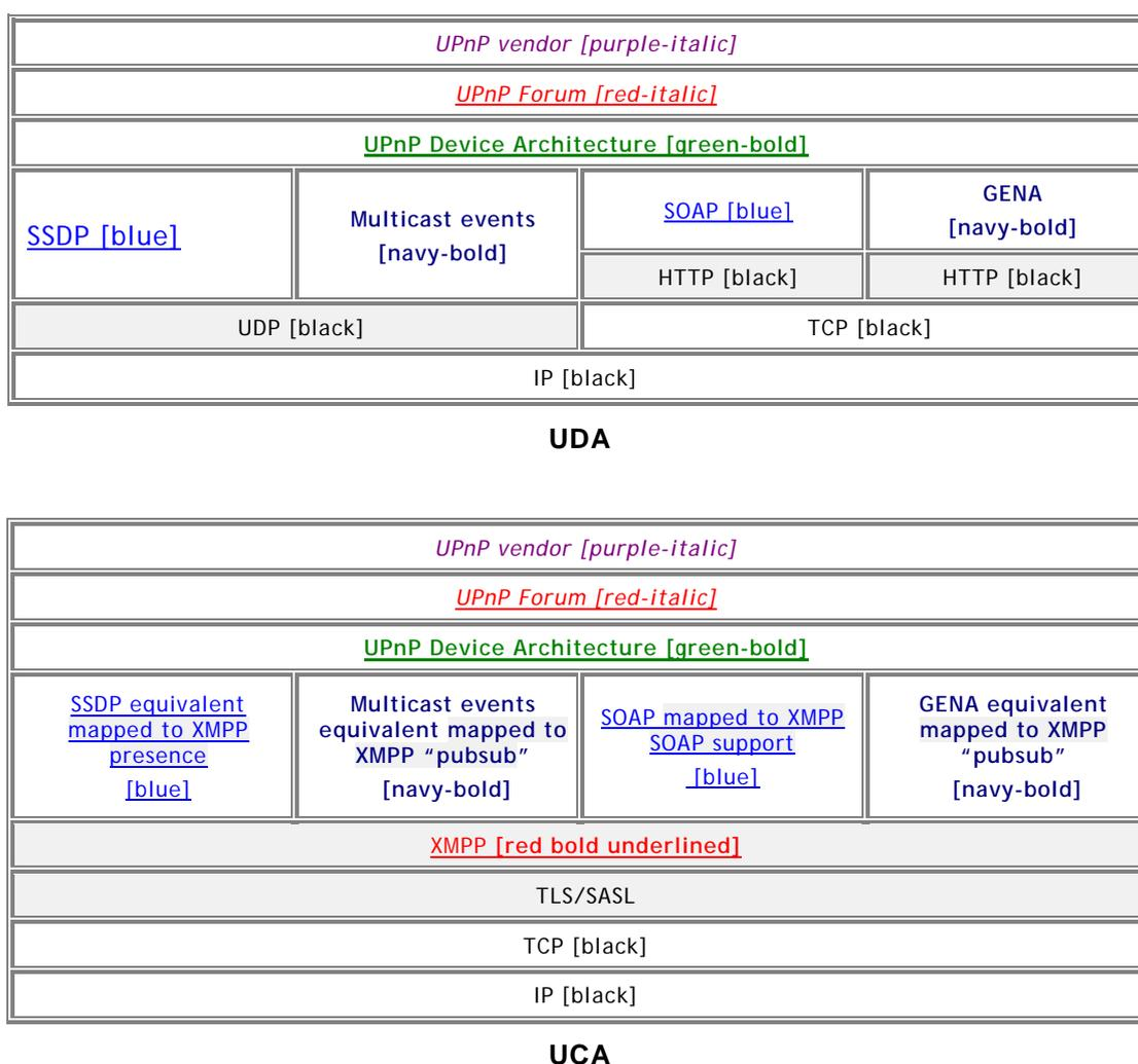
Figure C-2 provides a more detailed description of the UCA protocol stack. In this figure, two types of communication scenarios are illustrated. In scenario 1 (top) a UPnP Cloud Capable
