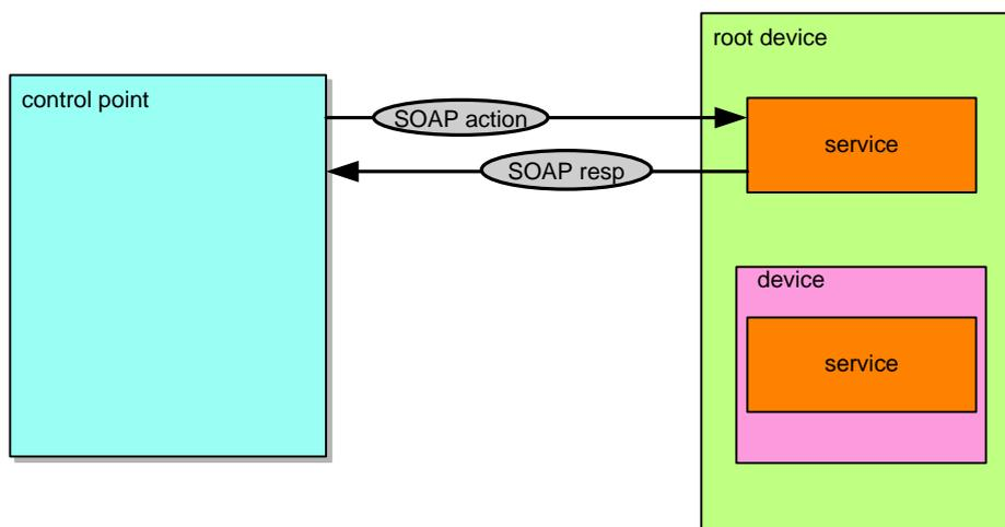
To control a device, a control point invokes an action on the device's service. To do this, a control point sends a suitable control message to the fully qualified control URL for the service obtained from the controlURL sub element of the service element of the device description. If the controlURL sub element is an absolute URL, the fully qualified control URL for the service is the controlURL sub element. Otherwise (the controlURL sub element is a
