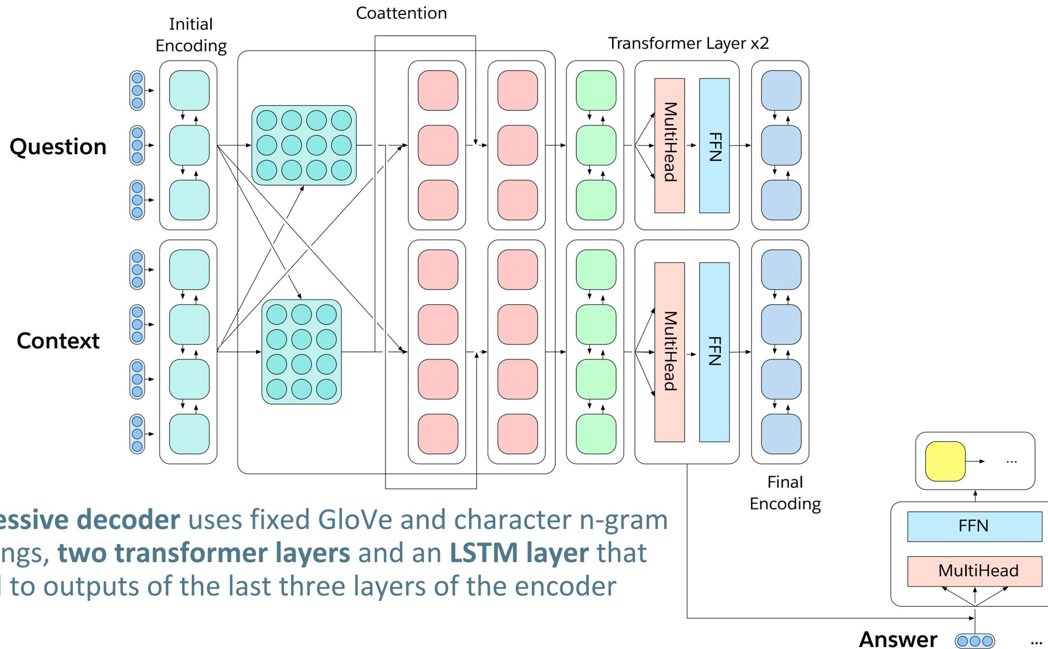
**Auto-regressive decoder** uses fixed GloVe and character n-gram embeddings, **two transformer layers** and an **LSTM layer** that attend to outputs of the last three layers of the encoder
