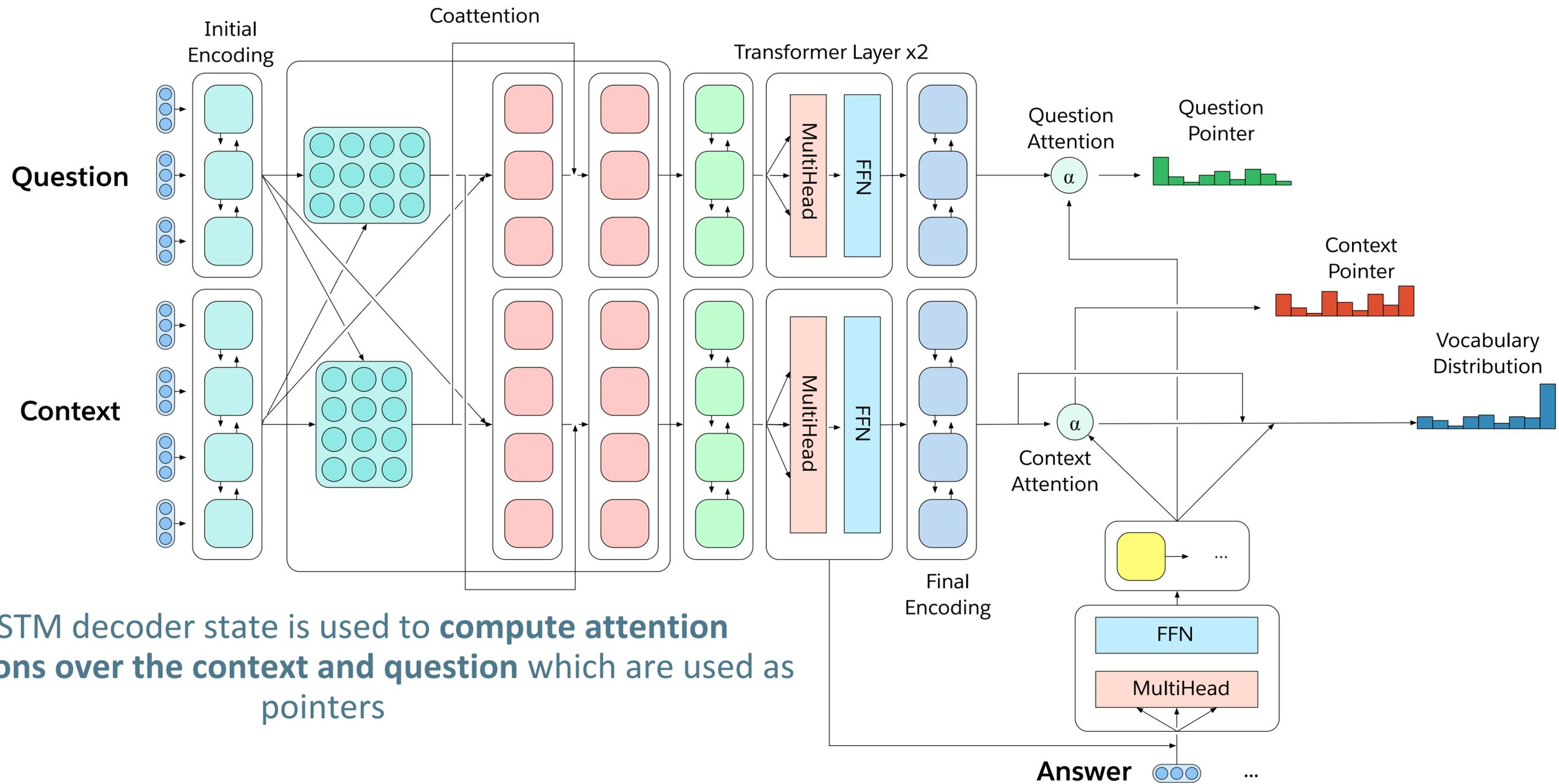
The LSTM decoder state is used to **compute attention distributions over the context and question** which are used as pointers
