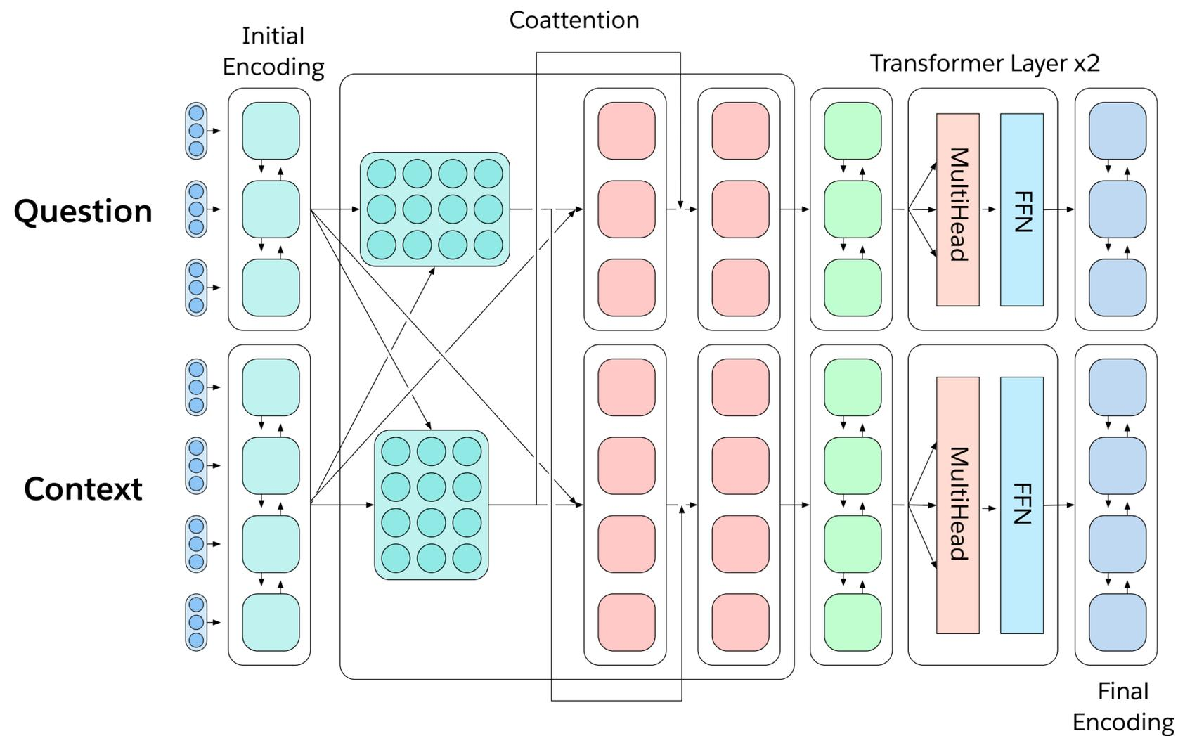
Separate BiLSTMs to reduce dimensionality, two transformer layers, another BiLSTM
